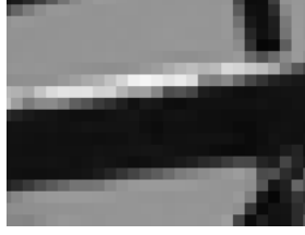
Fig. 1. Close-up of a horizontal edge. Note that the grayscales in the horizontal direction are quite smooth and thus can be well approximated using polynomial models.
